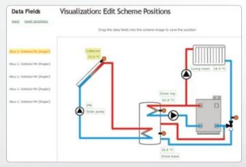
**Live Schemes:** Show your live data values in front of a schematic image of your solar system. Simply drag and drop the element to position it on the image on the right.
